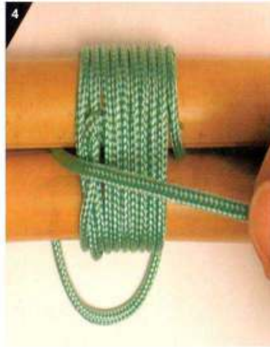
STEP FOUR. BRING THE ROPE UP BETWEEN THE POLES AND MAKE TWO TIGHT TURNS PARALLEL TO THE POLES.
