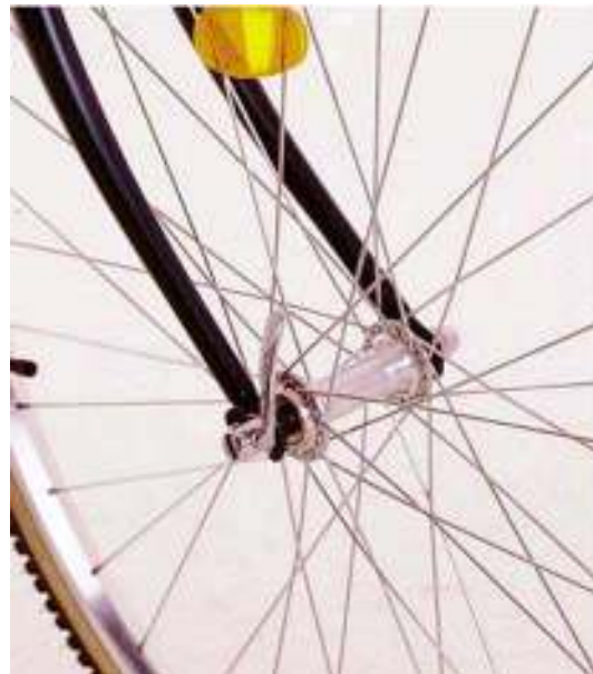
Figure 16-3-7 Quick Release Incorrect Position – Example 1
