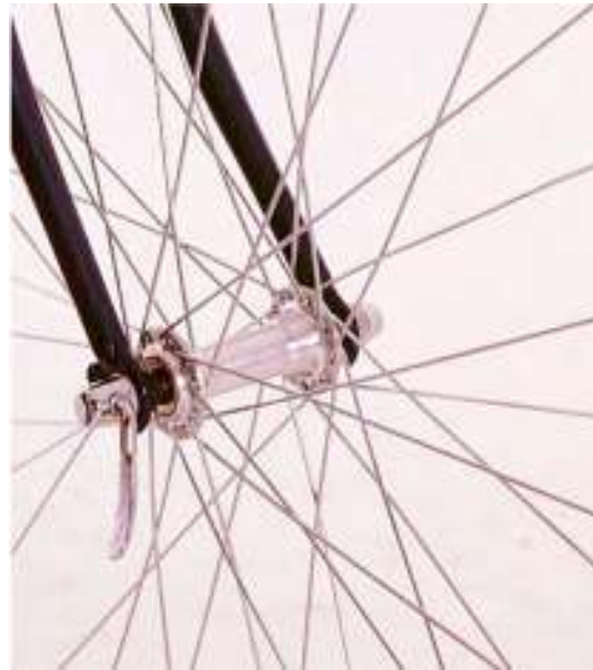
Figure 6 Quick Release Incorrect Position—Example 1
