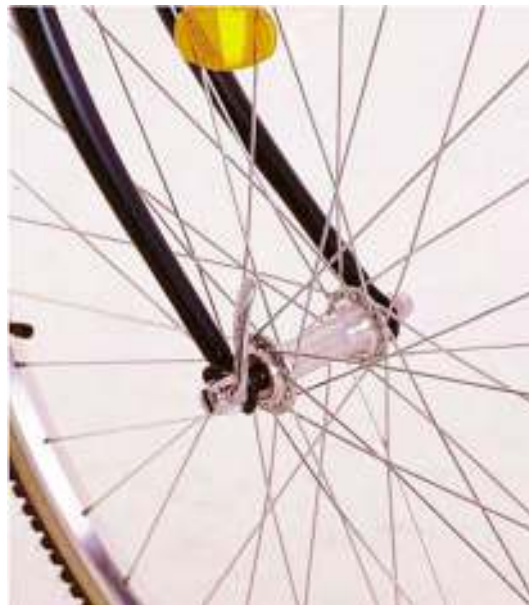
Figure 7 Quick Release Incorrect Position—Example 2
