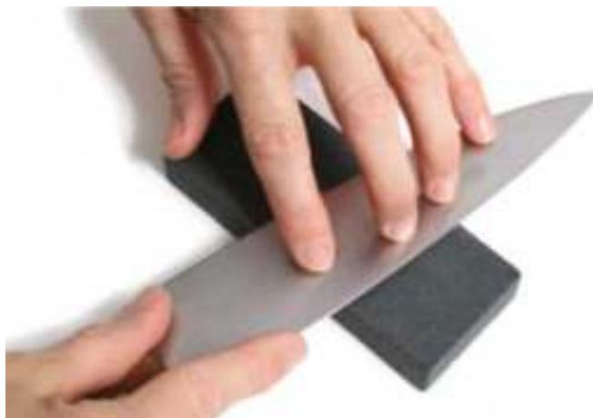
Figure 15 Sharpening the Reverse Side of the Knife
