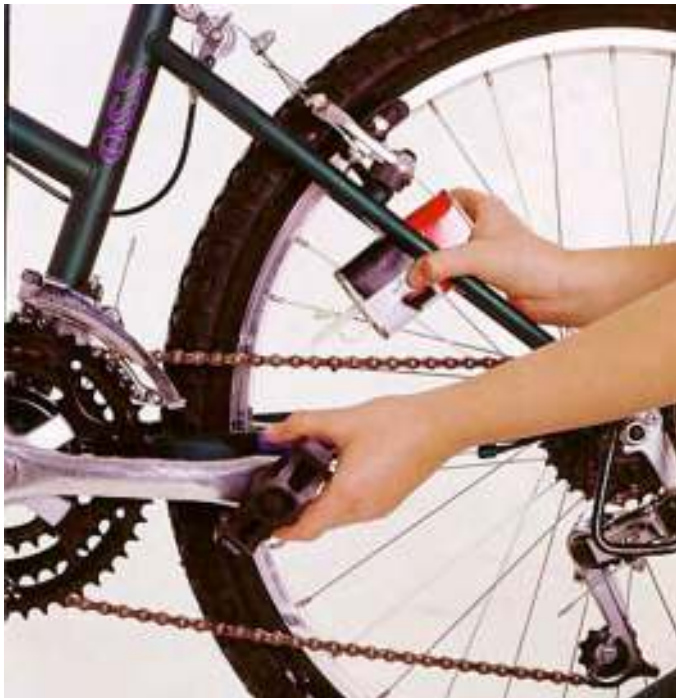
Figure 5 Lubricating the Chain
