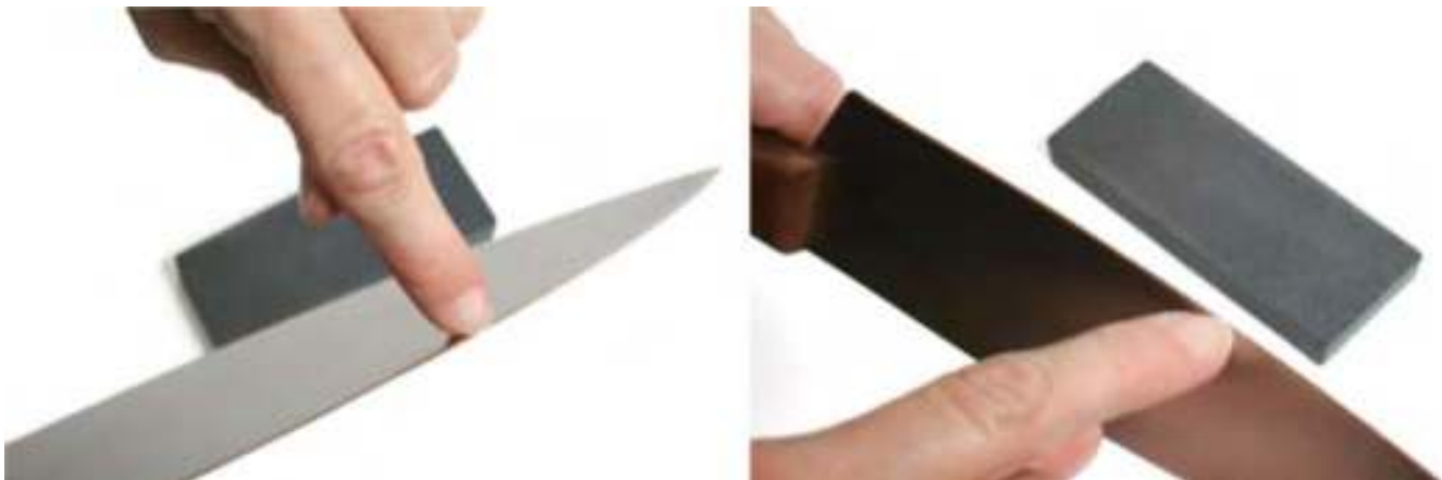
Figure 14 Checking the Bevelled Edge
